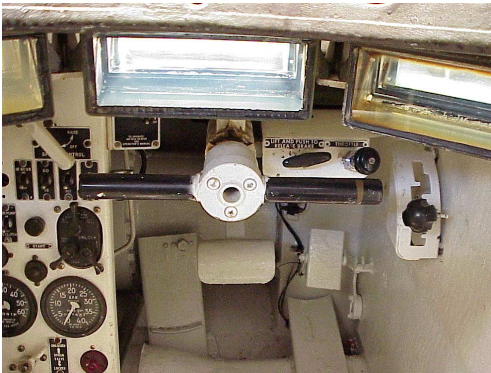
Fig III.4 - US M58 Driver's station, showing the steering yoke. The yoke used in this vehicle is actually an abbreviated steering wheel, which pivots about the roll axis. Unlike wheeled vehicles, in which several turns of the wheel may be needed for precise steering control, modern tracked vehicles are steered by differentially controlling their sprocket output shafts. Therefore, only limited rotation of the control device is needed. Elimination of the rim of the wheel allows more driver legroom, and eliminates obscuration of the instrument panel.
