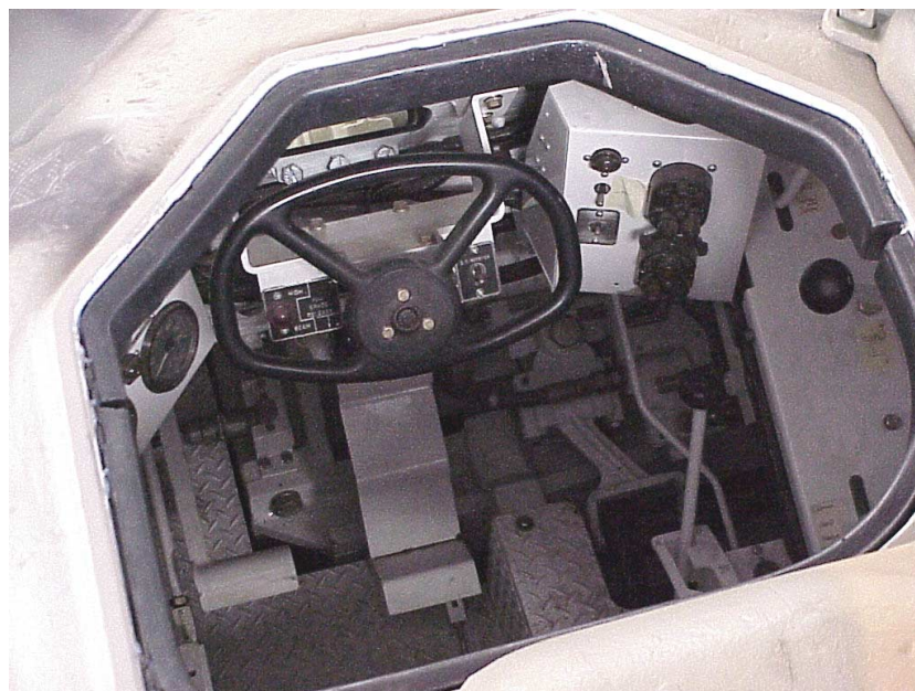
Fig III.6 - Driver's station in a US M88 recovery vehicle. The elliptical wheel has its axis offset to provide additional kneeroom for the driver. The operator frequently stands up in this vehicle to judge clearance, and needs to be able to reach the wheel from a standing position.
