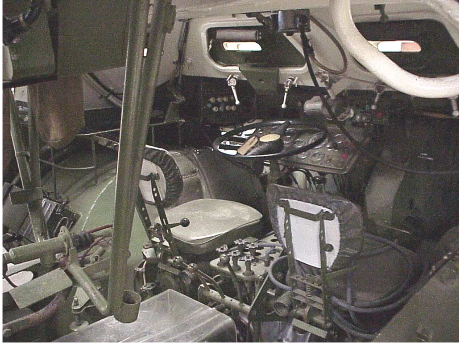
Fig III.3 Driver's station, showing the steering wheel used for directional control of this Russian wheeled APC.
